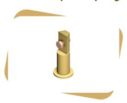
Cast Rod to tape coupling are copper alloy, Used in conjuction with the air rod brackets to connect the air rod and tapes. The coupling is screwd onto the air rod and then connects to the tape with the bolts.
