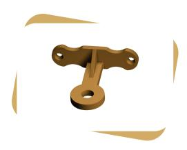
Rod brackets are copper alloy, These are being used for providing projection from the building wall or face. Rod breackets are mainly used with rod to tape coupling where it is not possible to fit a saddle on the roof and the air rod has to be fitted on the side of the building.
