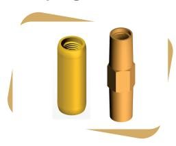
Coupling are copper alloy made of high grade Silicon Bronze, Aluminium Bronze and Brass for high streangh with counted bore for protecting the rod threads from damage. Also available ROUND & HEXAGON
